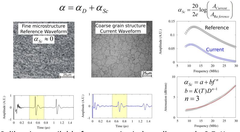
✓ Calibration available for austenite in low alloy steel: S.E. Kruger et al., Iron Steel Technol, (2005), 2(10),25
