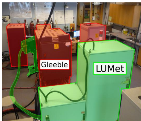
Fig.1: Gleeble3500 at UBC with LUMet system consisting of optical cabinet (in front) and the sensor attached to the Gleeble
